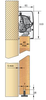
**RENOVATION, EXISTING DOOR FRAME**: Base you choice on the widht of opening existing to determinate the width of the door you use
