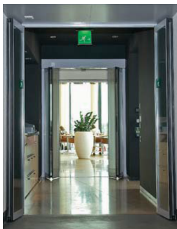
Automatic folding sytem where no space for sliding
